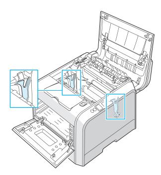
6 Hold the handle on the imaging unit with the green roller facing you. Align the imaging unit with the slots in your printer so that the colors on both sides of the imaging unit slide into the corresponding colors of the slots.
